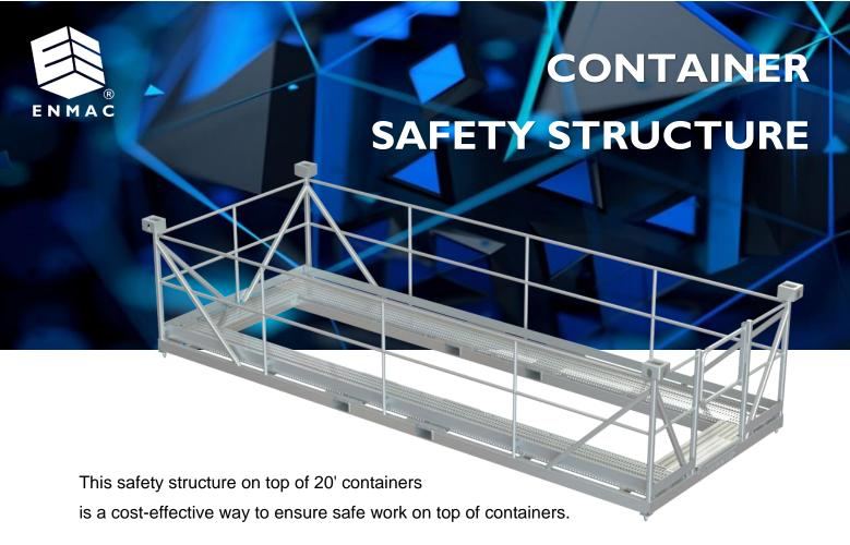
The safety structure is lifted onto the container with a forklift or crane. Due to the fixed corners, many safety structures can be stored on top of each other.
